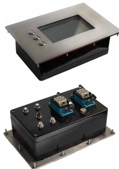
Rys. 6. Panel operatorski PO-1 [7]
